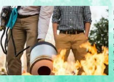
Firefighting with sound, also known as "acoustic fire extinguishment," is a concept that involves using high-intensity sound waves to control or suppress flames. The idea is to disrupt the flame's combustion process by applying specific frequencies that can disturb the airflow or heat transfer within the fire.
